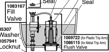
1083167 Fill Valve<br>85307 Washer<br>1057941 Locknut<br>42398 Washer<br>42397 Nut<br>1018165-A Gasket<br>1014065 Attachment Plate<br>1069722 (for Plastic Trip Arm) Flush Valve<br>1086115 (for Metal Trip Arm) |
