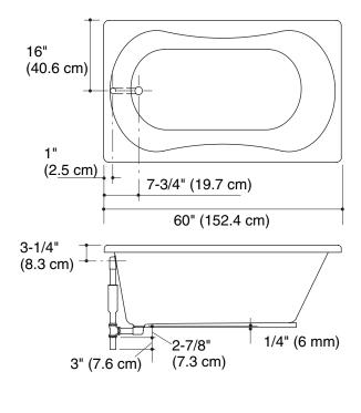
No change in measurements if connected with drain illustrated. (K-11677 or K-11677M)
