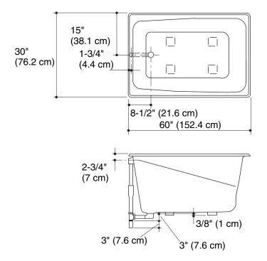
No change in measurements if connected with drain illustrated.
