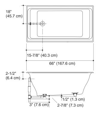
No change in measurements if connected with drain illustrated.
