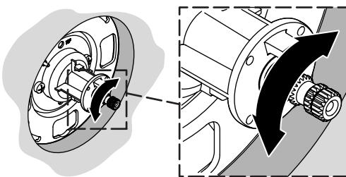
**18** Reinstall the collar with the setscrew against the tab.
