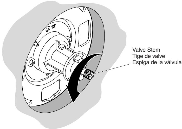
**21** Place the faceplate onto the valve and secure with the two screws.
