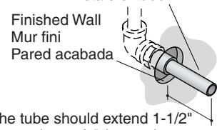
The tube should extend 1-1/2" (3.8 cm) - 2-7/8" (7.3 cm) past the finished wall.
