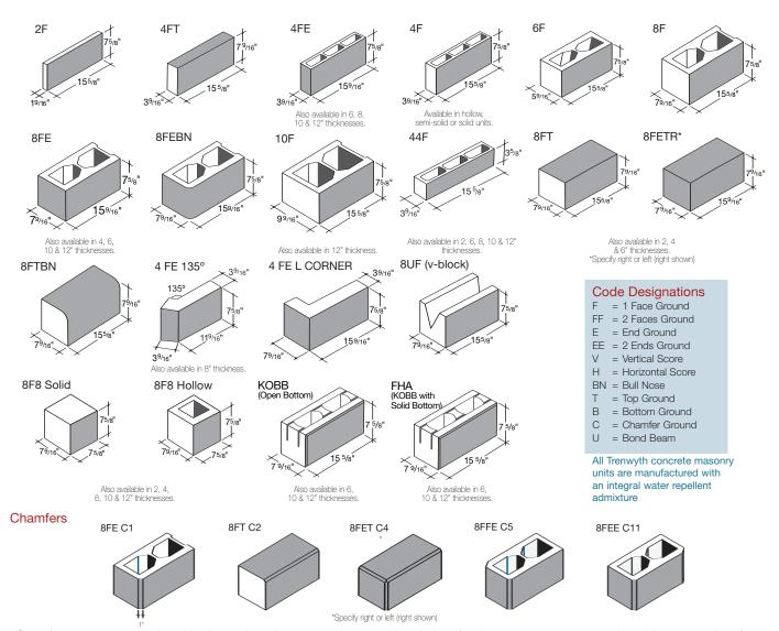
Chamfered corners minimize chipping and eliminate sharp corners. Not all chamfer designations are shown. Any side can be chamfered.
