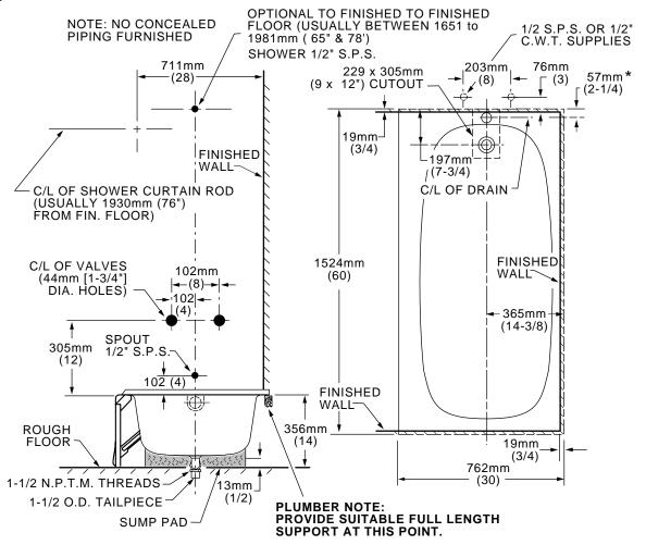
LEFT HAND TUB IS ILLUSTRATED. RIGHT HAND TUB IS REVERSED.
