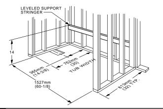
Position bathtub within the recess, check level, front to back, side to side. Also check drain clearance hole in sub floor. To secure the tub, use roofing nails immediately above the rear flange of the tub.
