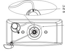
Locate bottom portion of hose clip between the ribs (2) on bottom of funnel inlet.
