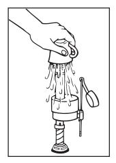
While holding a container over the uncapped VALVE to prevent splashing, turn water supply on and off a few times. Leave water supply off.
