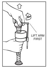
IMPORTANT: Always clear sand and rust from system. Make sure water supply is off. Remove valve TOP by lifting arm and rotating top and arm 1/8 turn counterclockwise, pressing down slightly on cap.
