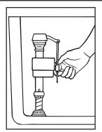
Turn on water supply. Adjust water to water level specified in the tank by squeezing water level adjustment clip and moving FLOAT CUP up or down along stainless steel link.
