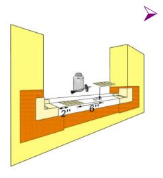
The spacers/supports must be installed at 6" on center starting 2" away from the corner pieces.
