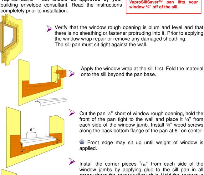
window jambs by applying glue to the sill pan in all areas where the corner will touch it. Hold the corners in place for 30 seconds or longer until they stay in place.
