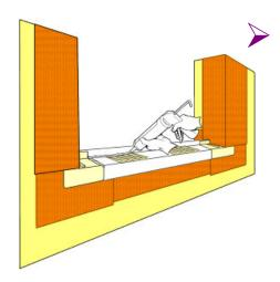
Prior to window installation run a bead of approved caulking (1 part Polyurethane) along the back upturned leg of the sill pan and over the pan-corner-joint. Push the window into the caulk for an air tight seal.
