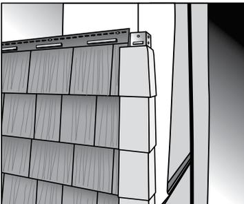
Hook the corner piece over the siding, making sure it engages into the starter strip and nail through the top two holes.
