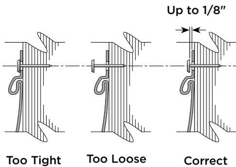
**NOTE: Do not nail too tightly. To permit expansion and contraction, panels should hang freely from nails. This allows the panels to move as the temperature changes. Drive the nails until there is between 1/8" to 1/16" of space between the nail head and the nailing flange.**
