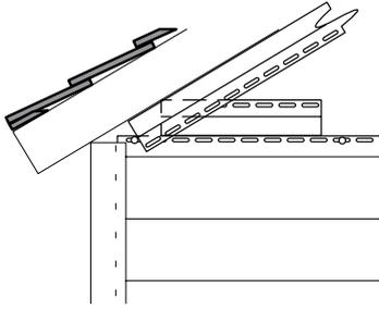
To create an angle template, hold a piece of J-Channel against the slope while transferring the angle to another J-Channel with a pencil.
