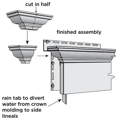
Cut the crown molding cap in half. Apply each half to the end of the crown molding and secure it with a bead of caulk.
