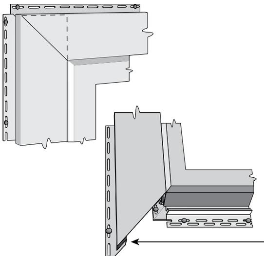
Snap the completed top lineal into the previously attached starter strip. Bend the rain tabs of the top lineal down into the receiving pocket of the side lineals.
