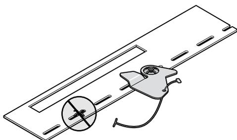
You must install the cam clip and the snap rivet at the same time. Installing the rivet before the clip may cause the rivet to mushroom and prevent it from keeping the cam clip securely in place.
