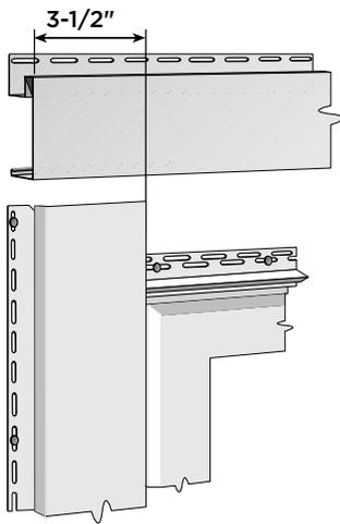
Measure the top of the opening and add 7" if the side lineals are also 3-1/2" (3-1/2" extra for each side equals 7"). Add 10" when using 5" lineals.
