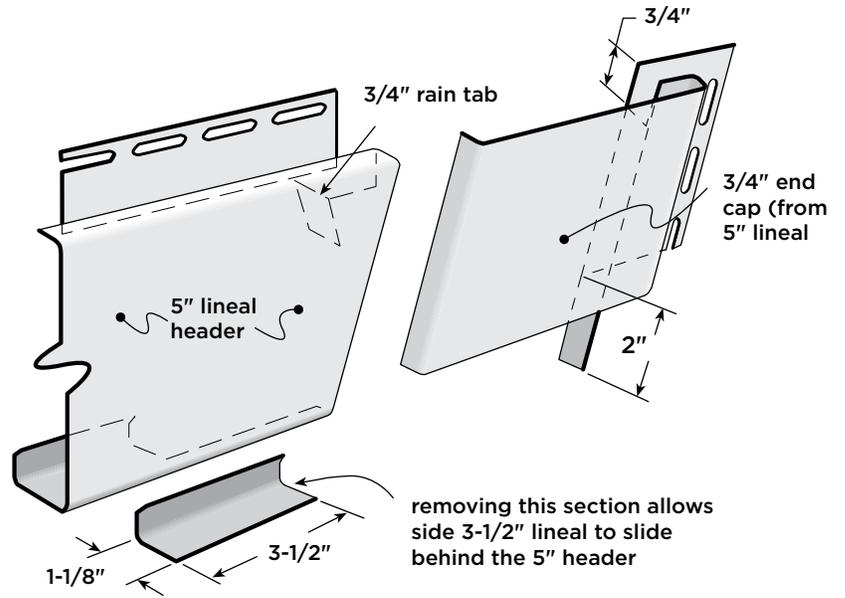
Finish the corner by sliding the 3-1/2" side lineals behind the header, making sure the 2" rain tab on the end cap extends into the receiving area of the side lineals.
