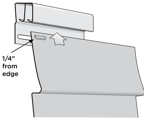
To install, lock the bottom of the cut panel into the panel below. Push the top edge into J-Channel or undersill trim. Tabs will catch in the trim and hold the panel firmly in place.
