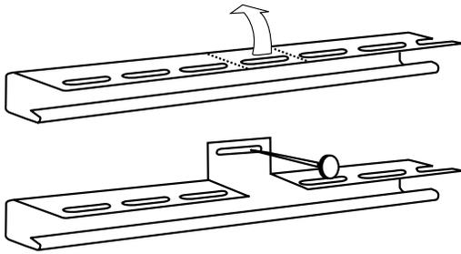
**NOTE:** If you don't have the proper receiver for the soffit, you can modify J-Channel to create an F-receiver. Simply cut slots in the nail flange area where the receiver will be nailed to the wall, bend back the flange, and nail the flange to the wall.
