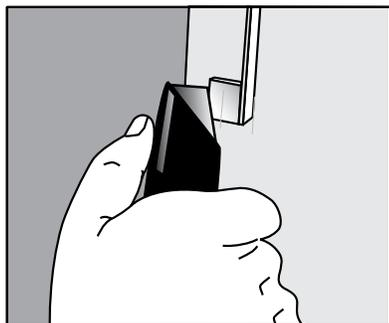
Flip the panel over and cut 1/8" off the side locking tabs.
