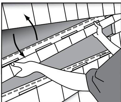
**NOTE:** To eliminate interference from the panel above the damaged panel, use two roofing nails as a wedge to prop up the upper panel.
