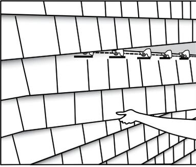
Place the heavier part of the cam clip up against the cam. While applying pressure to the top panel, pull down on the thinner end of the clip.
