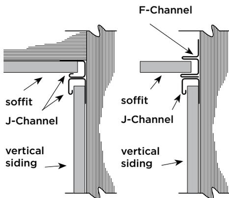
Install inverted J-Channel along the top of the wall, under the eave. Here again, leave a 1/4" gap between J-Channel and cornerposts. Overlap J-Channels 3/4" to allow for expansion. When positioning the upper J-Channel, be sure to allow for expansion of the siding panel. In most cases, position the J-Channel at a point equal to the length of the panel plus 5/8" (1/4" for upper expansion and 3/8" for lower expansion).
