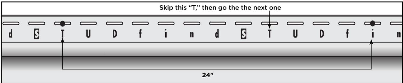
**NOTE:** Monogram XL 25' panels must be "center pinned" to control expansion and contraction. To do so, locate the center nailing slot of the panel and drive nails into both ends of the slot (see illustration). This is only done for one nail slot per panel.
