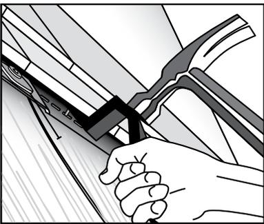
Lift up the panel above the new panel far enough to place the nails into the old nail holes.
