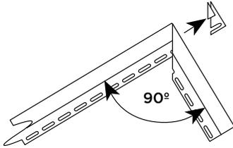
Next, transfer the angle of the template to the end of a length of J-Channel. Be sure to extend the line onto the nail flange. Cut away the channel face and the nail flange.
