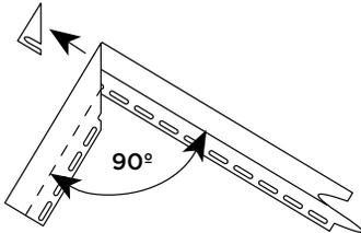
Turn the pattern over and transfer the opposite angle to the second J-Channel, being sure to extend the line onto the nail flange. Cut away the nail flange and return lip, but do not cut the J-Channel face.
