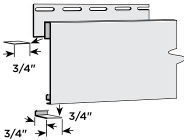
Notch both ends of the header as shown.
