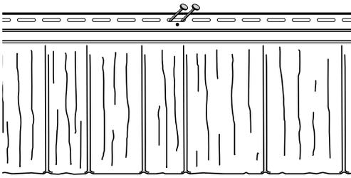
Locate the mark at the center of the panel. Use the nailing slot closest to this mark. Center pin the panel in this location using one of the following options:
