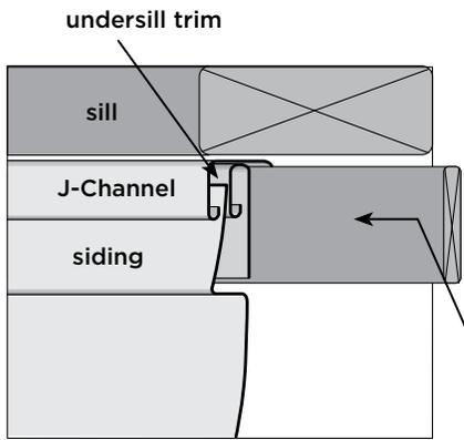
Furring and/or foam is also used below eaves and windowsills to maintain correct slope angles when siding panels must be cut to a narrower dimension to fit.
