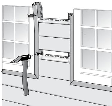
If the area is very narrow, leave one J-Channel unnailed except at the lowest point (as shown). Bend this channel out slightly to insert panel. When the panel is in place and nailed, nail the J-Channel immediately above the panel and repeat the procedure. Be sure to leave adequate tolerances for expansion and contraction.
