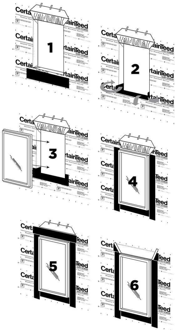
1. Make diagonal cuts in the weather-resistant barrier at the upper corners of the top (head) of the rough opening. Gently lift and tape the flap temporarily in place.
