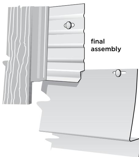
Lock the Cedar Impressions panels into the starter strip and secure it.
