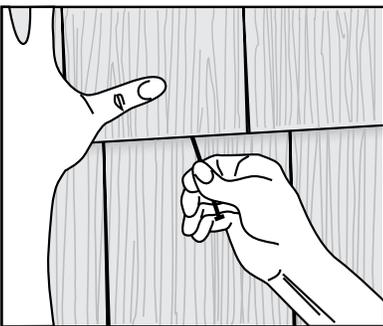
Using your wonder bar or roof snake bar, drive the nails in by placing the bar on the nail head and hitting the bar with a hammer.
