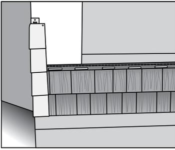
Angle the panel into the cornerpost and slide to the left until the side tabs clear. Next, slide the panel to the right until you have the correct temperature marks on the panel lined up.
