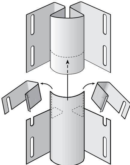
If you have to splice the inside cornerpost, cut 1" off all but the outer face of the lower post. Lap 3/4" of the upper post over the lower post, leaving 1/4" for expansion.
