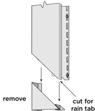
Use a triangle to create a 45° angle or measure 3-1/2" in from the locking leg.
