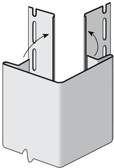
Lap the partial receiving channel of the new post over the partial channel on the remaining nail flange. Pop rivet the two receiving channel legs together as needed.
