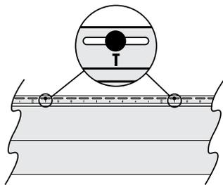
When installing CedarBoards XL 16'8" panels, the succeeding studs are at every 8th slot. When you apply the next panel, adjust the overlap, as necessary to line up with studs and repeat the steps above.
