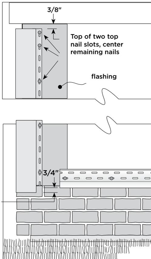
**NOTE:** If the transition material allows, the bottom 3/4" of the channels may be removed from the outside cornerpost so that the face of the corner may be positioned lower and more in line with the bottom of the siding. This method creates a transition with more pleasing aesthetics. The outside cornerpost face must still maintain 3/8" or 5/8" clearance from obstructions.
