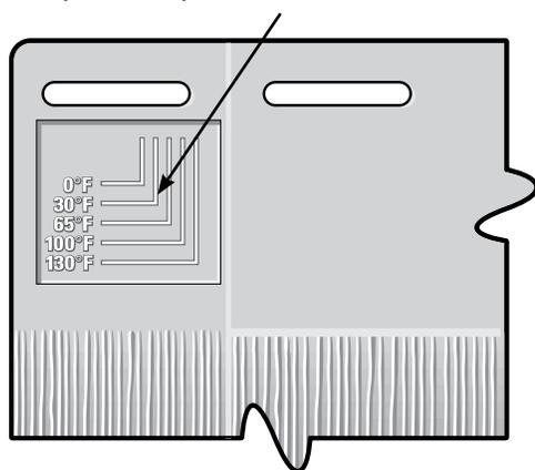
**PRO TIP:** When installing Cedar Impressions over foam insulation, extra care needs to be taken to verify that adequate space is left between all nail heads and the panel.
