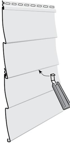
With a zip-lock tool, unlock the buckled panel from the panel below by inserting the hooked end of the tool behind the return leg of the buckled panel until the hook catches.
