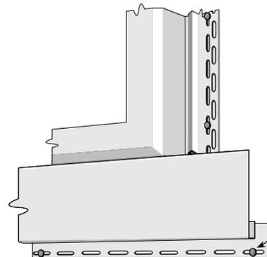
Snap the lineal in place and secure by nailing (or stapling) it through center of the nail slots.
