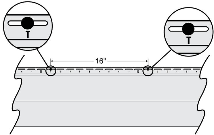
Standard 12' panels feature 10 nail slots every 16", with one of the 10 letters in the word "STUDfinder" centered directly under each slot. Locate the first stud and fasten the siding to it in the center of the nail slot. Notice which STUDfinder letter appears below the slot.
