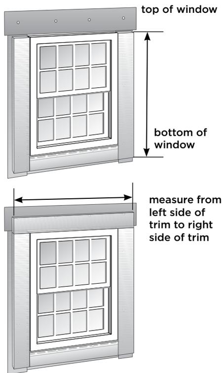
these pieces to the left and right sides of the window, verifying that the top edge of each section lines up with the top of the window and the bottom edge of each section lines up with the bottom edge of the first piece of trim already applied.
