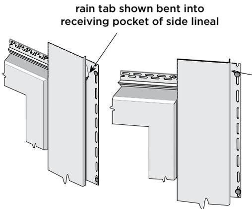
Snap the side lineals into place to check the fit.
