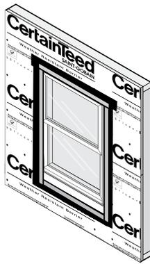
If installing a new window and flashing, refer to the window manufacturer's instructions and ASTM E2112, Standard Practice for Installation of Exterior Walls, Doors, and Skylights for the proper flashing installation method for the window type and wall configuration of the project.
