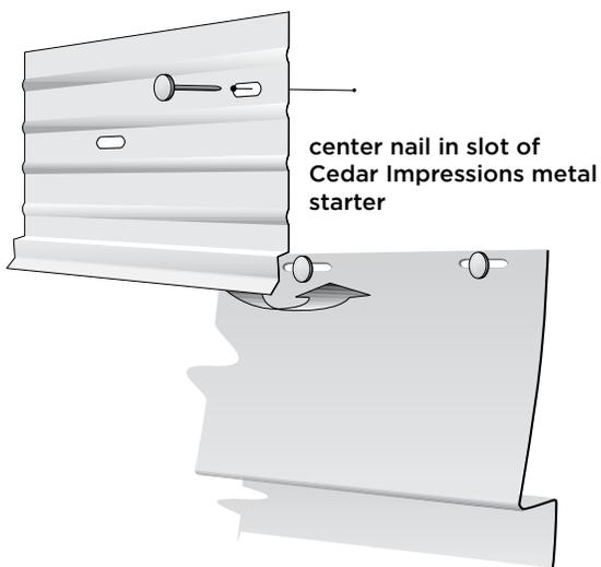
Secure Cedar Impressions 4" Metal Starter after hand punching and securing the siding piece.
