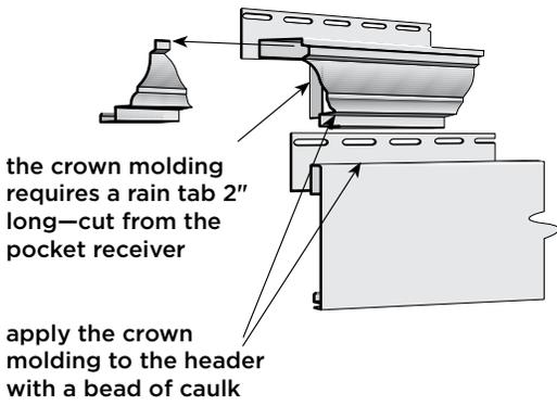
Insert a crown molding cap into the crown molding and trace the shape. Trim as shown.
