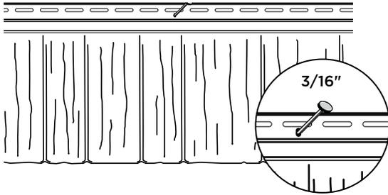
Apply fasteners at nail slots aligned with studs a maximum of 16" apart. Leave adequate room between the fastener head and the nail flange for expansion and contraction (approximately 1/16" to 1/8").
