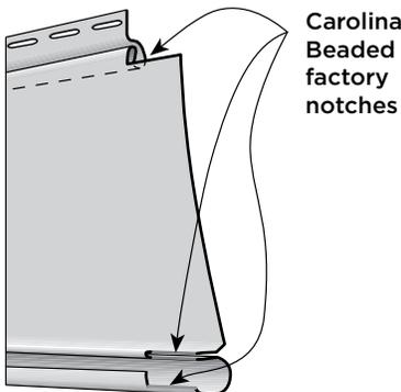
**NOTE:** The Carolina Beaded panel is factory-notched in three places. For best results, overlap panels using factory notched ends only. If a panel must be cut on site, insert cut ends into receiving channels in cornerposts or J-Channel. If this isn't possible, create an exact duplicate of notches using aviation or tin snips.
