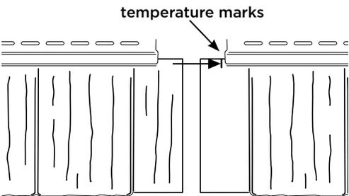
Install the next panel to the left of the installed panel. Lap this panel over the installed panel, positioning the right edge of the panel to the appropriate temperature mark, which is located in the factory notch area.
