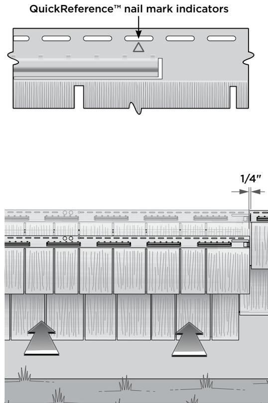
Install the next panel by positioning it below the starter strip and next to the first panel. Push in and up to lock the panel into the starter strip and the side tabs of the first panel. Space the second panel according to the panel temperature at the corresponding temperature indicator lines.
