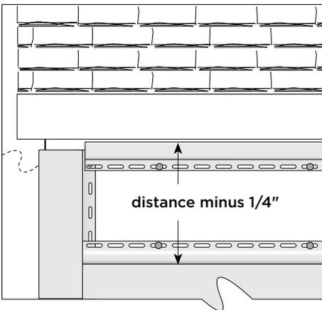
Measure from the soffit to the base of upper lock on the previous course of panels. Subtract 1/4". Mark this dimension on the panel to be cut, taking the measurement from the bottom edge of panel. For a more precise cut, repeat this procedure at several other points along the span to be covered by the panel.
