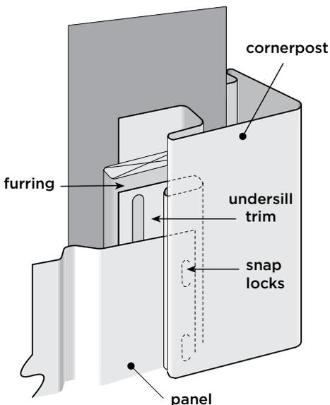
Using a level, make certain this panel is plumb. Nail every 12”. Follow the same nailing procedures described for horizontal siding.
