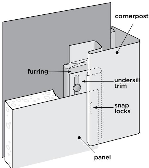
**NOTE:** When applying overlapping accessories, you may have to make new slots to avoid pinning the underlying accessory.
