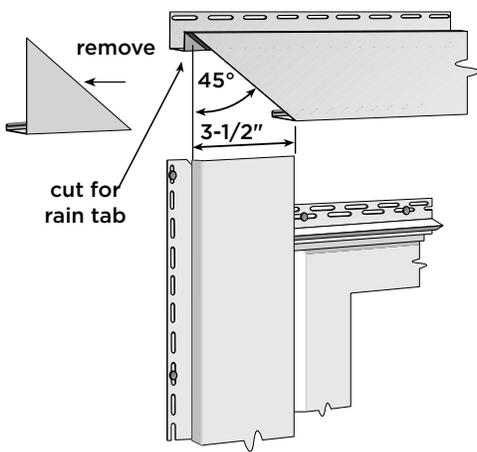
Use a triangle to create a 45° angle or measure 3-1/2" in from the locking leg.
