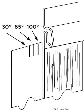
If the ambient temperature is less than 45°F, lap the panel to the first (30°) mark.
