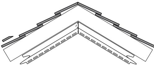
Insert the full-faced J-Channel into the mitered J-Channel. If the nail flange or return lips butt and prevent a tight fit, trim off additional material from the second J-Channel.
