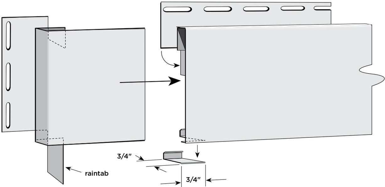
**NOTE:** To make end caps for 3-1/2" lineals, simply start with a 5-1/2" piece and remove the 3/4" and 2" areas as shown for the 5" end caps.
