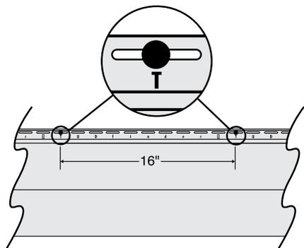
Locate the first stud and fasten in the center of the nail slot. Ensure that nail penetration is at least 1-1/4" into framing members to comply with ASTM D4756 (specification for vinyl siding installation). Notice which STUDfinder letter appears below the slot.
