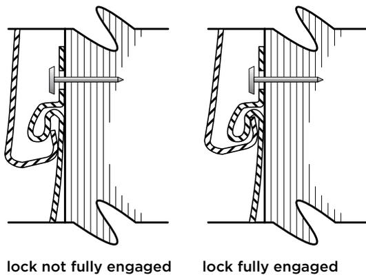
Slide the first panel into the cornerpost recess. Leave room for expansion (see page 37-38 for spacing requirements).
