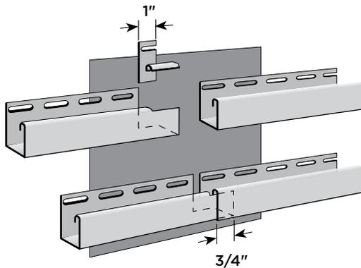
Install inverted J-Channel along the top of the wall, under the eave. Here again, leave a 1/4" gap between the J-Channel and the cornerposts. Overlap the J-Channel 3/4" to allow for expansion. When positioning the upper J-Channel, be sure to allow for expansion of the siding panel. In most cases, position the J-Channel at a point equal to the length of the panel plus 5/8" (1/4" for upper expansion and 3/8" for lower expansion).
