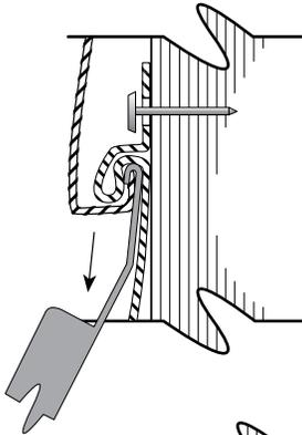
Insert an inverted scrap piece of starter strip into the exposed receiving lock of the lower panel.
