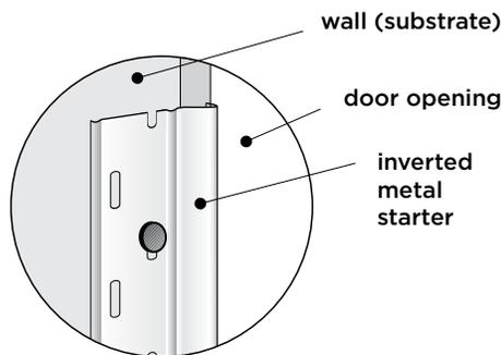
If the opening has no framework, such as a brick molding, use the metal starter in place of the Window and Door Starter Strip. The lineal's locking leg will fit behind the aluminum starter and into the receiving pocket of the Window and Door Starter.
