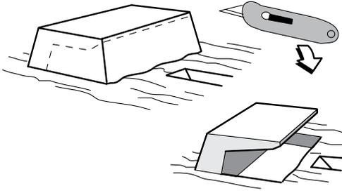
Another look can be achieved by using the lower locking tabs. First, remove the protective material from the sides of the tabs (see left). Lock the upper panel into the tab and secure.
