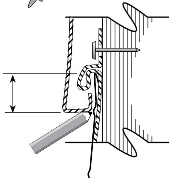
Trim the starter on this line, saving the portion with the locking edge.
