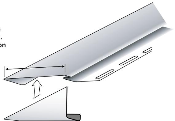
Using PVC cement primer and cement on both pieces, slide the part into the lineal to create an assembly.
