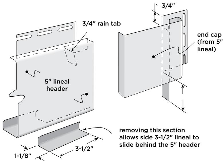
Finish the corner by sliding the 3-1/2" side lineals behind the header, making sure the 2" rain tab on the end cap extends into the receiving area of the side lineals.
