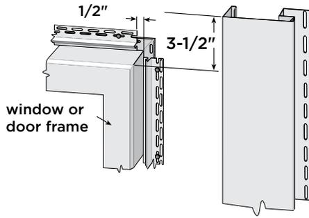
Measure the height of the window. Add 7" if using 3-1/2" lineals for the header and bottom lineal. (When using 5" lineals at header, add additional material). Cut lineal to length.
