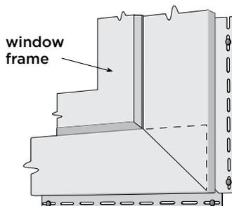
Snap the side lineals into place and secure using nails or staples.
