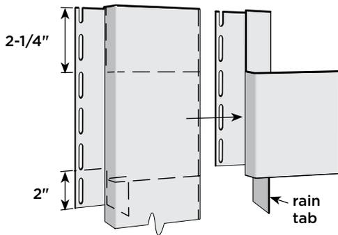
To create the header end cap, cut a 9-1/4" piece of 5" lineal and trim as shown.
