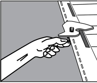
Push on the back button of the snap rivet to secure the clip to the panel. Repeat over each locking tab area.
