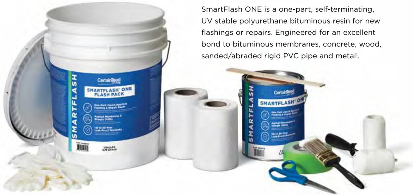
SmartFlash ONE is a one-part, self-terminating, UV stable polyurethane bituminous resin for new flashings or repairs. Engineered for an excellent bond to bituminous membranes, concrete, wood, sanded/abraded rigid PVC pipe and metal<sup>1</sup>.
