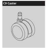
2<sup>1</sup>/<sub>2</sub>-inch-diameter doublewheel caster; black nylon wheels and yoke; soft polyurethane tread; internal brake; for use on hard floors or carpet
