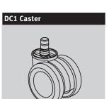
2<sup>1</sup>/<sub>2</sub>-inch-diameter doublewheel braking caster; black nylon wheels and yoke; for use on hard floors or carpet; quiet roll technology
