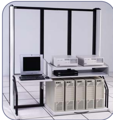
▲ Components mount directly to the face of the frame and can be precisely positioned on the frame along a one-inch vertical standard. Components fully engage the frame via mounting tabs or "hooks" and are easily relocated using common tools.
