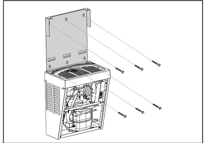
5. Set bottle filler onto the basin. Feed the power cord and 3/8" water line through hole in the basin.
