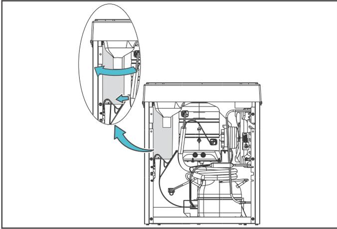
5. Check all the lines and connections for water leaks. Repair connections if necessary.
