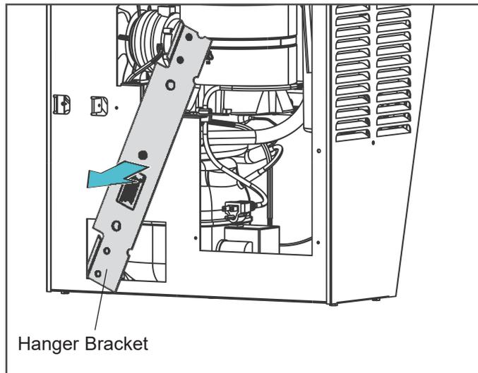
3. Install the hanger bracket with five screws in 7/16" diameter mounting holes.
