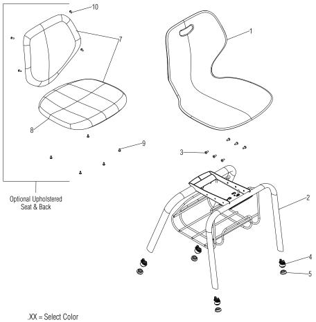
Item 2 replacement frames do not come with glides. Glides must be ordered seperately. Item 6 felt glide (used after 2011), uses caps that are replaced when worn.
