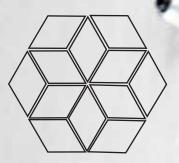
Configurate's shared-edge design allows electrical connection between each module. This interface between the modules is installed on site. Linked together, the configuration connects to the relevant number of remote drivers. The inherent modular nature of the system allows for ease of change during the design or installation stage by adding or removing modules.
