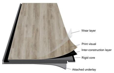
Figure 1: Diagram of rigid core flooring cross section
