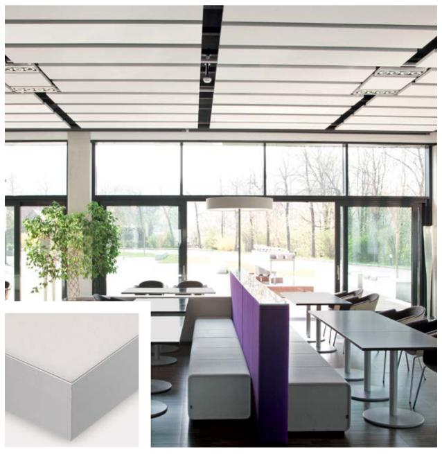
BALANCE and BALANCE PLUS Ceiling Clouds provide acoustical control while maintaining the appearance of an open ceiling. Completely preassembled, BALANCE products are easy to suspend from any ceiling or roof deck and are ideal for open office environments and loft spaces.
