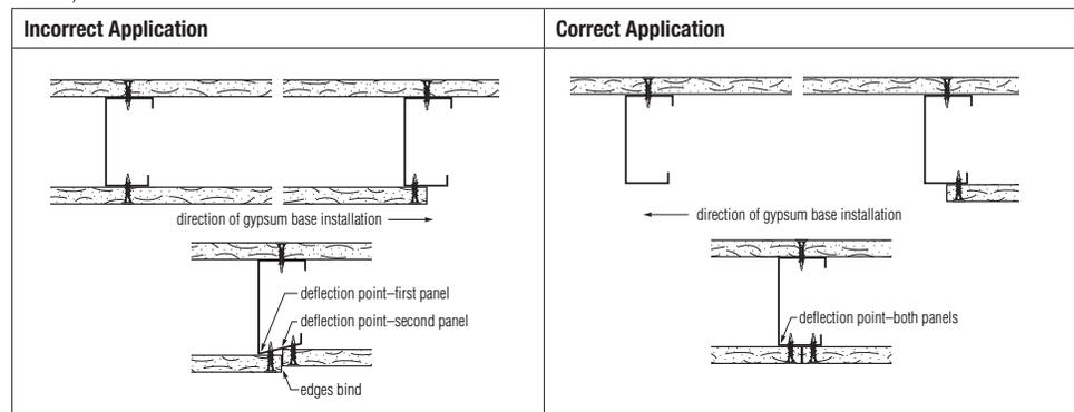
Lipped or stepped joints from improper framing or base installation will result in distortion of the joint area and an unacceptable finished wall.
