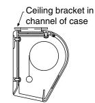
To mount against ceiling, hold screen case against ceiling and mark mounting hole locations. Each bracket has two holes towards the front edge and two holes towards the back edge. Installer must use at least two fasteners per bracket with one fastener in one of the two holes closest to back edge of bracket, and one fastener in one of the two hole closest to front edge of bracket. Installer must insure that fasteners are of adequate strength and suitable for the mounting surface chosen.
