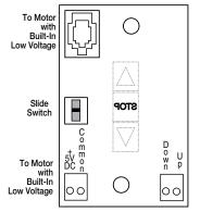
Please Note: 5V DC must be connected to be able to set limits using the wall switch.
