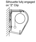
Engage the lip on back of screen case with lip of "Z" Clip and gently pull down to fully engage case to brackets.
