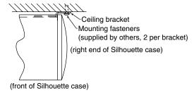
To mount suspended from ceiling, the brackets need to be installed on screen case as noted on page 1. Use "S" Hooks through the holes in the brackets to attach to ceiling. Select the set of holes that allows the screen to hang in a vertical position. The installer is to provide the "S" Hooks and the materials and fasteners to attach the "S" Hooks to the ceiling. Installer must insure that the fasteners and suspension material is of adequate strength and suitable for the mounting surface chosen.
