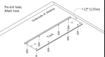
Note: Orient track so holes align with channels on Series 9000 top.
