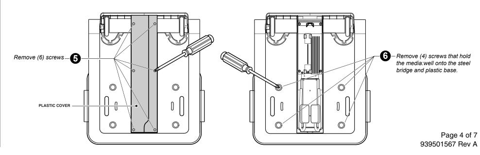
**7.** a) Remove (6) screws from the media:well, then b) remove the bezel.
