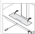
Flip-up door in base provides easy access to a power and data cables storage compartment.
