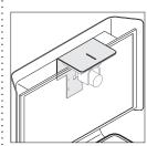
**Under-mount camera ledge** accommodates most industry standard HDVC cameras. Depth is 8" and width is 11½".
