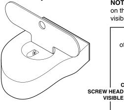
**NOTE:** The cam pin is offset and needs to be installed on the shorter offset side. If the screw heads are not visible, turn the panel/shelf 180°.
