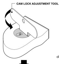
Use mallet, before tightening cam screws, to bring parts together and avoid light leaks.
