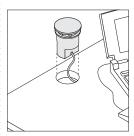
**Port** is field installed. Use a 3½"-diameter drill to cut mounting hole at desired location.
