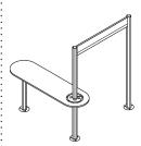
"L" configurations with capsule worksurface must use large foot and be attached to the floor. Consult with project's architect or structural engineer to determine floor construction and proper attachment hardware.
