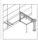
For Montage applications with a combination of panel-mounted and tethered or freestanding worksurfaces with legs, the worksurface(s) supported by legs will not reach the same height as the cantilevered worksurface if panel glides are extended more than ¼". Standard Montage worksurface height is 28%" H when panel glides are at zero. Legs adjust up to 287%" H.
