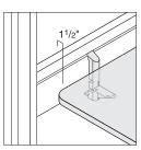
**Gap** between beam and table is 1½" and allows cords and cables to drop behind the table.
