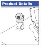
Power and communication spheres are field installed. Use a 3"-diameter drill to cut mounting hole at desired location.
