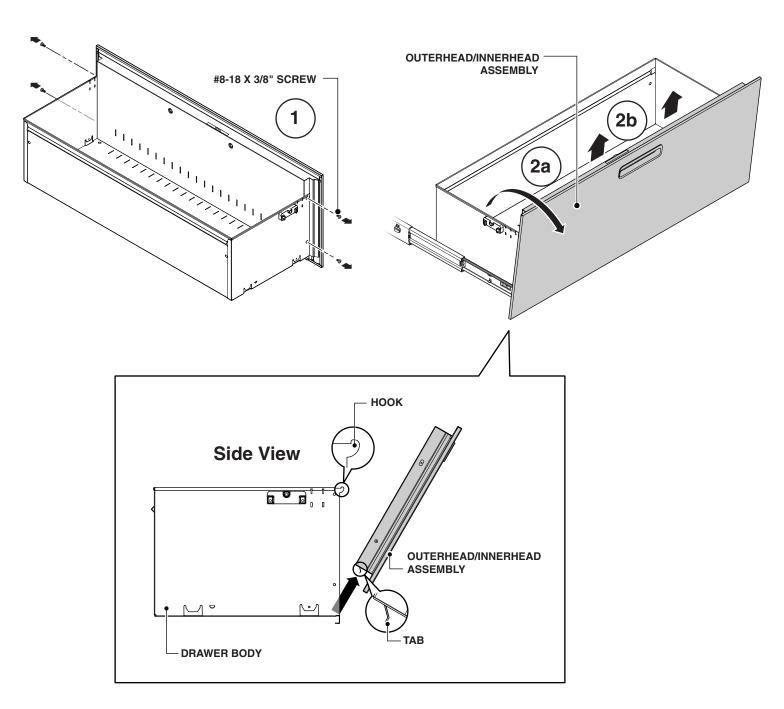
Removing the Innerhead from the Outerhead Assembly
