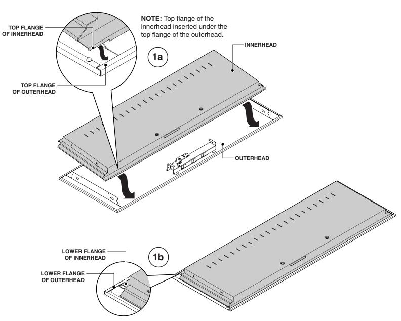
**NOTE:** Flex the lower flanges on the innerhead to bring it above the lower flange of the outerhead.
