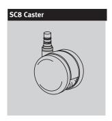
21/2-inch-diameter double-wheel caster; black nylon wheels and yoke; soft polyurethane tread; quiet roll technology; for use on hard floors or carpet
