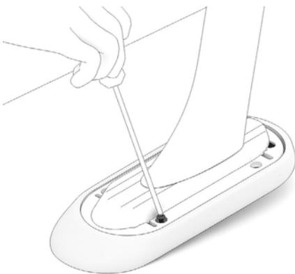
12. Using T-20 torx driver remove arm pad screws (4 screws for adjustable pad, 1 screw for fixed pad).
