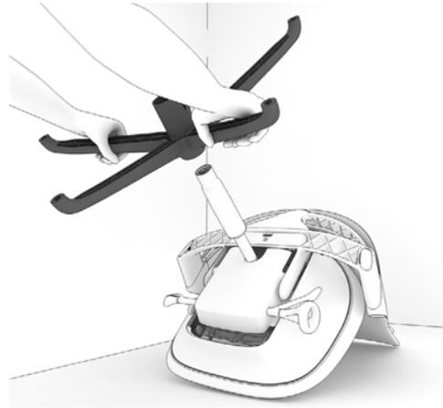
4. Disengage the base from cylinder.
