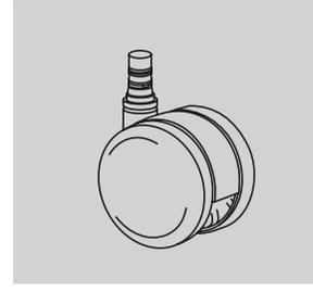
2 1/2-inch-diameter double-wheel medium roll-resistant caster; black nylon wheels and yoke; soft polyurethane tread; for use on hard floors or carpet; quiet roll technology
