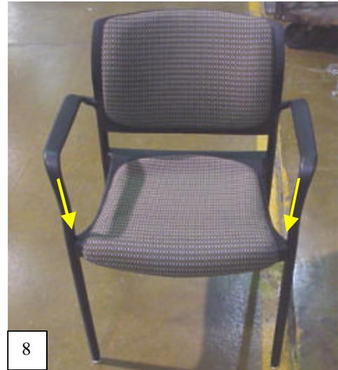
When both left and right arms are in position, slide the backrest and arms down onto the frame tubes, towards the seat. When the backrest and arms are pushed all the way onto frame, turn the arms 90° towards the seat of the chair. The arms will not rotate if the backrest and arms are not pushed all the way down onto the frame. Push the front end of the arms in the tubes located in front of the frame.
