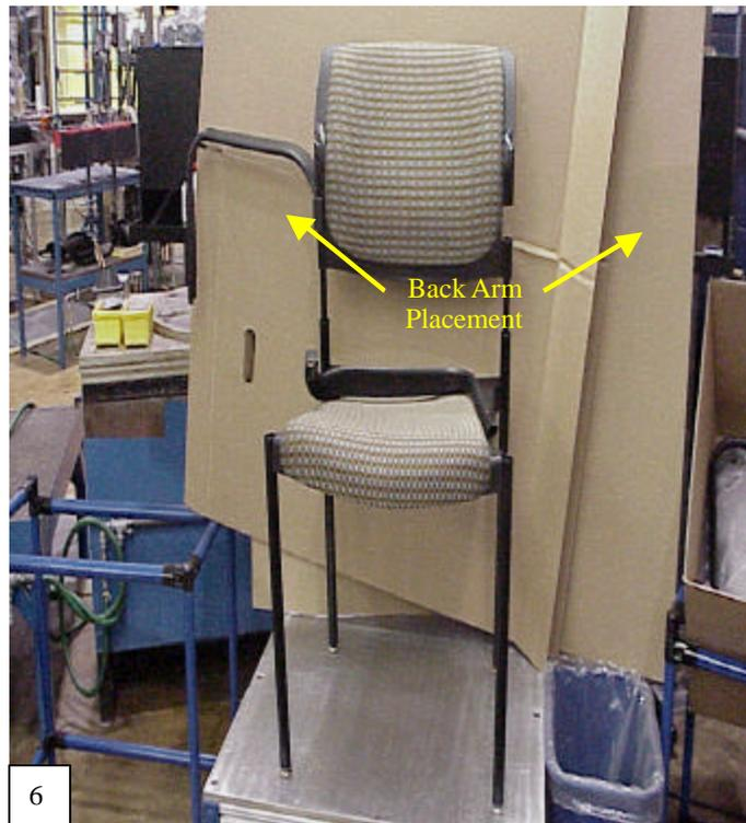
Slide the new backrest down onto the frame until the frame tubing comes up to the bottom of the arm cutout area on the backrest. Put the back of the arms in the cutout areas with the arms turned sideways 90° from the chair assembly.
