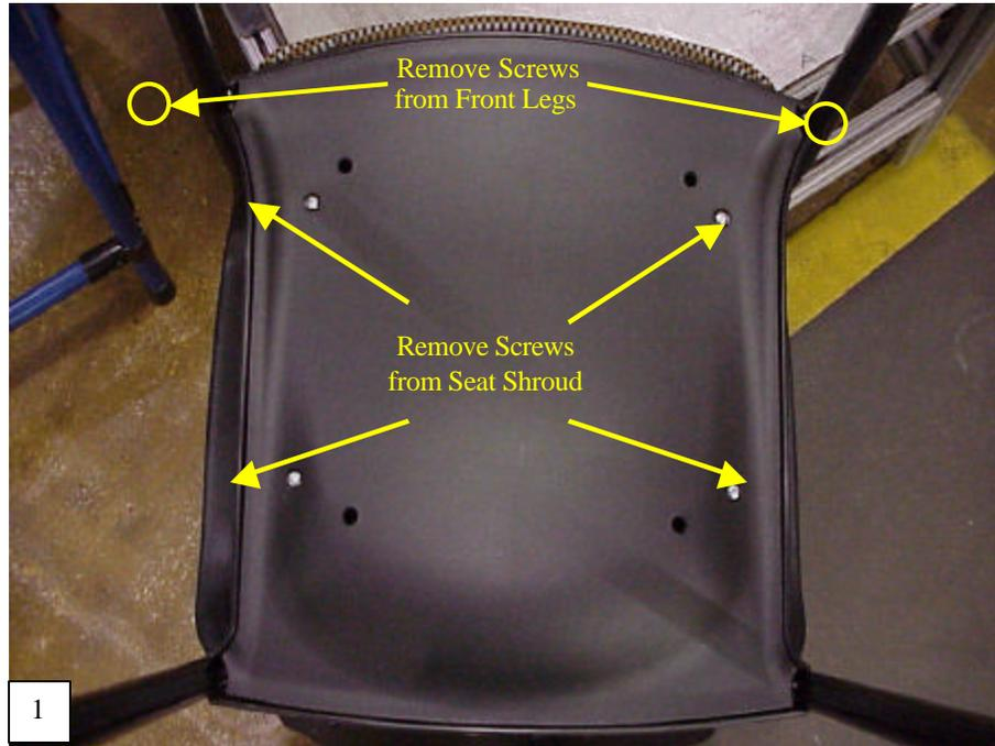
Turn the chair upside down and place the seat on the corner of a table. Using a Phillips screwdriver bit, remove the four screws in the seat shroud. Next remove the seat shroud from the chair assembly. Now remove two arm screws, one screw in each of the front two legs. Turn the chair back over to the upright position.
