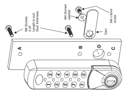
DIAMETER 4.5 / 5.0mm **DIAMETER 16.0 / 16.5mm** USE EITHER OR BOTH OF HOLES B & C **ALWAYS USE FIXING HOLE A** HOLES A, B & C HOLE D
