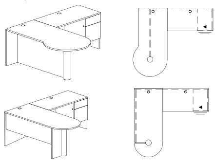
A suspended P- or D-Top is mounted to the front edge of the adjoining surface.
