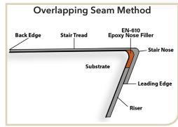
When overlapping stair tread and riser seams, ensure that the stair tread and riser have been trimmed and fit the step snuggly. Risers do not normally require trimming on the top edge prior to installation when overlapping seams. However, if the top edge of the riser extends up to or over the height of the step, trim riser to 1/4" - 1/2" from the top of the step to allow space for the EN-610 Epoxy Nose Filler Adhesive.
