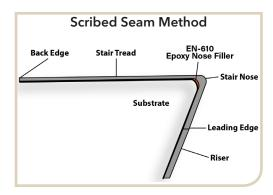
When butting stair tread and riser seams using the Scribed Seam Method, ensure that the stair tread above and below the riser, as well as the riser itself, have been trimmed and fit the step snuggly. Ensure the stair tread below the riser is in place prior to scribing the riser to ensure a tight fit to the leading edge of the stair tread above.
