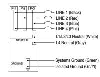
NOTE: L-4 should alternate between P-1, P-2, and P-3 to balance circuit loading.
