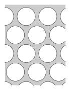
Round-1/2" perforations  $0.600^{\prime\prime}$  o.c., 63% open area not to be used with the USG Curvatura™ One-Directional Ceiling System
