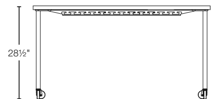
Side Elevation of Desk Height, with Casters
