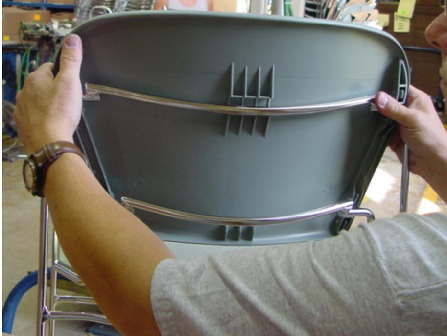
**Step 6.** Take the new back panel and snap it into the front panel by aligning the slots on the top and bottom portions of the back. The top portion must be snapped under the upper lip of the front panel indicated by the yellow ellipse.
