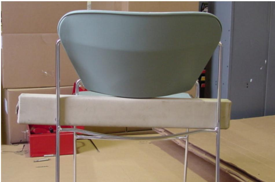
**Step 3.** With the cordless driver and T15 bit, back out all 4 screws that hold the back together. Note if a 2x4 is not available, 2 people are required. One person to flex the back and the other for screw extraction.
