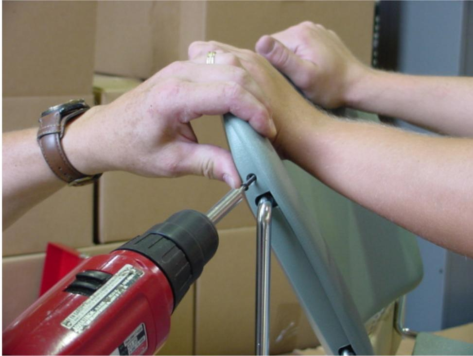
**Step 4.** Remove the 2x4 if used. Separate the 2-piece back by prying at the bottom portion of the front panel and pulling forward.
