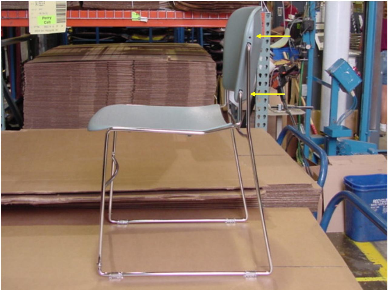
**Step 2.** The back must be in the flexed position to gain access to the bottom two screws in step 3. Two options are available to achieve this:
