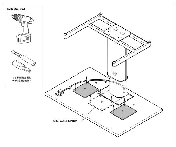
Choose your own locations for the two (2) weight plates and mount with four (4) #10 x 1" pan head wood screws per weight plate.
