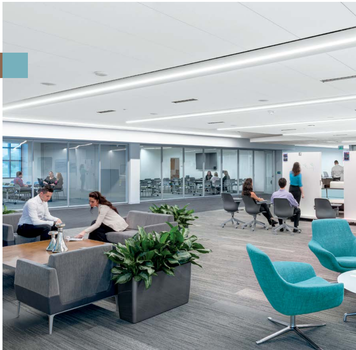
Ultima® 24" x 48" Tegular panels with Suprafine® 9/16" suspension system. Running bond pattern is achieved by using XTAC clip.
