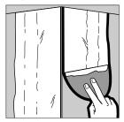
Using a 6" taping knife for outside corners (4" for inside corners), apply another coat of joint compound (Easy SAND, Topping, All-Purpose, or Lightweight All-Purpose). Keep this coat as smooth as possible. Feather out 5" to 6" (125 to 150 mm) from the nose of the trim on each side for outside corners (1" or 25 mm past previous coat for inside corners). Let dry. Sand sides lightly where needed.
