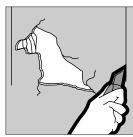
b. Slip drywall repair clips onto the edge of the damaged wall. Position screws about 3/4" in from the edge and centered between the tabs. This will line up the screws with perforations in the clips. Screw through wall into each drywall repair clip.
