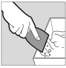
While embedding tape, draw the knife slowly along the length of the tape to provide an even distribution of joint compound. Don't worry about a few grooves or streaks in the joint compound. They will be covered over in the subsequent coats.
