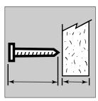
Drive nails in straight, not at an angle. Do not overdrive or countersink nails. This results in breaking the face paper or fracturing the gypsum core. If a nail happens to go in crooked, hold the panel tight against the framing and drive a second nail in about 2" from the nail that punctured the paper. Then drive the first nail in below the surface of the board.
