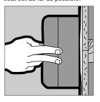
When applying earlier coats, minor depressions and grooves were not a problem. However, do not leave any during the application of this final coat or they will mar the finished surface.
