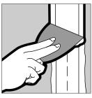
To reinforce tapered joints, follow same procedure. Tape should overlap tape applied to butt joints.
