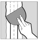
While embedding the tape, remove excess joint compound from edge and apply as a thin coat over the tape.
