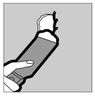
b. Crisscross two or three strips of joint tape over opening and embed tape in joint compound. Let harden.
