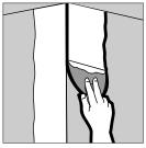
Place trim on wall and press into position. Corner bead should be aligned tight to ceiling. Embed trim by running the knife over it with even pressure at a 45° angle.
