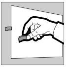
**5 Torn Gypsum Panel Face Paper** a. Peel and remove loose face paper.
