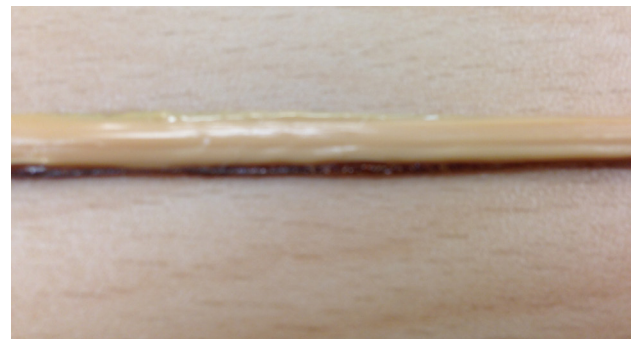
Example of a heat welded seam that has been burned. The heat welding gun may have been too hot for the pace the operator was moving.
