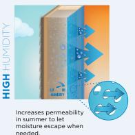
MemBrain can adapt from fully closed to open (<1 to 35 perms) to provide greater drying capability.
