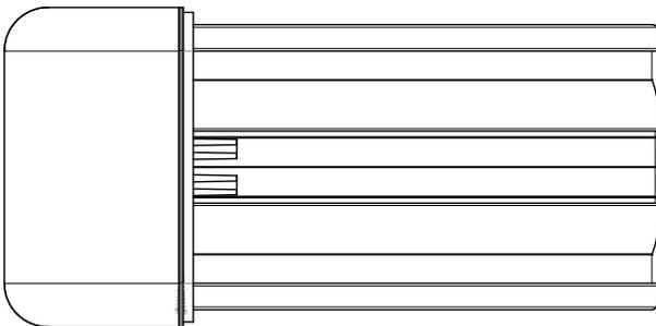
2. Attach Returns and Corners to retainer, leaving 1/16" gap between Return/Corner and retainer allowing for adjustment. **See Fig. 3.**
