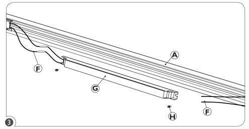
Disconnect the power wires (F) from the ballast (G). Unscrew nuts (H) and disconnect ballast (G) from fixture (A). Replace ballast (G) and reconnect to fixture (A).
