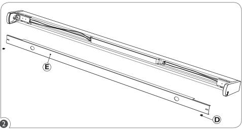
Unscrew the ballast cover retaining screws (D) and remove the ballast cover (E).
