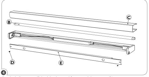
Put the ballast cover (E) back in place and fasten retaining screws (D). Re-install the lamp (B) and lens (C).
