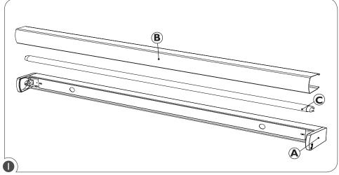
**NOTE:** Ensure that the power to the fixture's circuit is turned off before attempting to verify and replace the ballast. Remove lens (C), and the lamp (B) if installed from the fixture (A).
