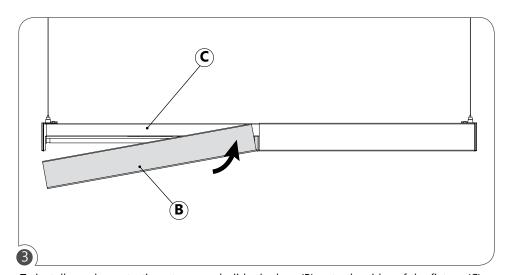
To install new lens, starting at one end, slide the lens (B) onto the sides of the fixture (C).
