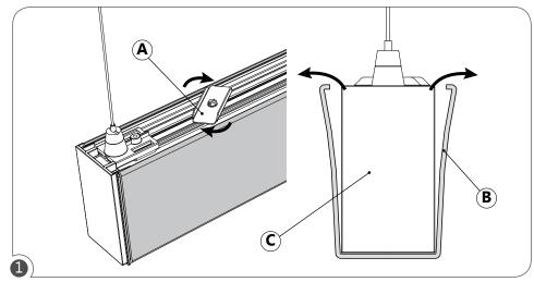
Turn the lens clip (A) to release the lens (B). Pry both sides of the lens (B) away from the fixture (C) at one end.
