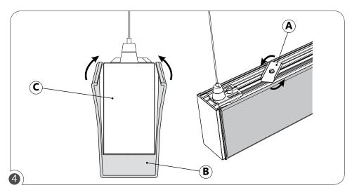
Pushing the lens (B) onto the fixture (C). The lens (B) will snap into it's final place. Turn the lens clip (A) to lock the lens (B) in place.
