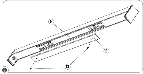
Remove ballast cover retaining screws (D) and remove the cover (E) to reveal the ballast (F).
