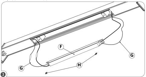
Disconnect wires (G) from the ballast (F). Remove the ballast retaining nuts (H). Replace ballast (F) and reconnect wires (G). Re-install the ballast into place and fasten retaining screws.
