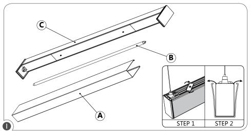
**NOTE:** Before attempting to verify and replace the ballast, ensure that the power to the fixture's circuit is turned off. Remove lens (A) by unlocking the lens lock. Remove the lamps (B) from the fixture (C).
