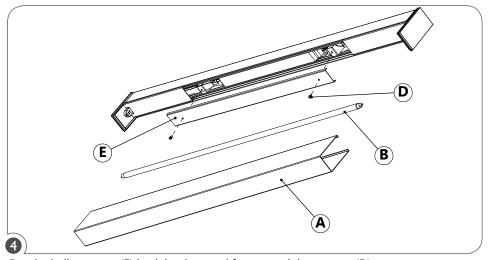
Put the ballast cover (E) back in place and fasten retaining screws (D). Re-install the lamps (B) and lens (A). Lock the lens in place using the lens lock.
