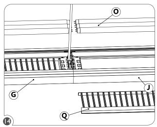
Install the lamps (O) in the fixtures. Reinstall the optics (Q) back to the second fixture (J).
