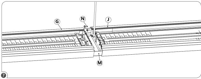
Connect the second fixture (J) using the aligner (M) and secure with screws (N).
