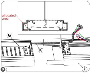
Push the electrical wires (K) from the first fixture (G) through the second fixture (J) in the allocated area on the side of the extrusion.
