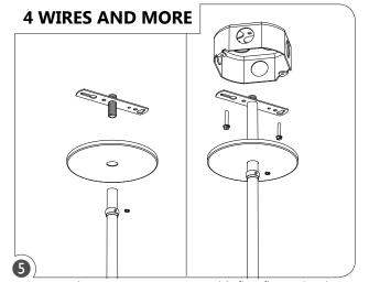
For a continuous row systems: With first fixture in place, repeat steps **1** and **4** for the next fixture in line.
