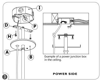
On the power side, raise the fixture to the ceiling and make electrical connection using wire nuts (P). Secure with screws (H) the j-box crossbar (D) to the junction box (I). Slide the canopy (B) and secure in place with the trim ring (A).
