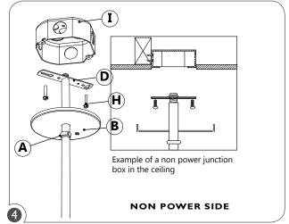
On the non power side, raise the fixture to the ceiling and secure with screws (H) the j-box crossbar (D) to the junction box (I). Slide the canopy (B) and secure in place with the trim ring (A).
