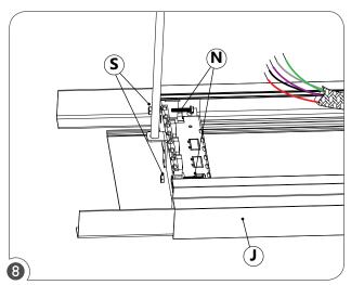
Remove the joinning screws (N) and nuts (S) and set aside for later use.
