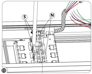
With the joinning screws (N) and nuts (S) from step (8) join both fixtures together.
