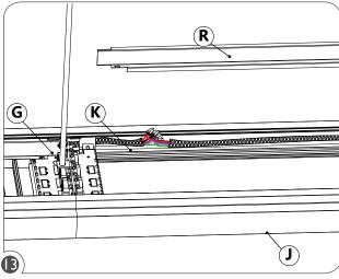
Push the electrical wires (K) into the side of the extrusion and screw the reflector (R) back to its place.
