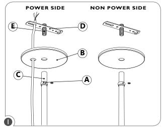
Slide the trim ring (A) and then the canopy (B) onto the stem (C) and leave loose. Screw the j-box crossbar (D) with the <sup>3</sup>/8" threaded stud (E) onto the stem.
