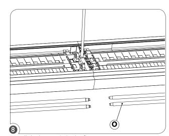
Install the lamps (O) in the fixtures.
