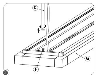
Screw the stems (C) onto the threaded bracket (F) at the ends of the fixture (G).
