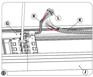
Connect the electrical wires (K) from both fixtures using the supplied quick-wire connectors (L).
