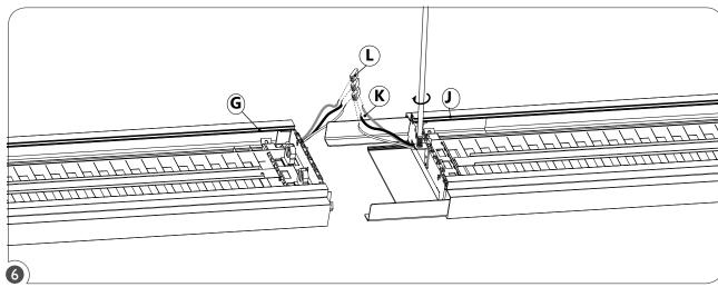
Connect the electrical wires (K) between the two fixtures (G) and (J), using supplied quick-wire connectors (L).
