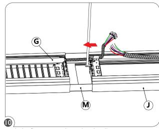
Push the fixtures together using the aligners (M).
