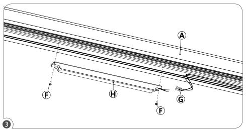
Remove the ballast retaining screws (F). Disconnect wires (G) from the ballast (H). Replace ballast (H) and reconnect wires (G).
