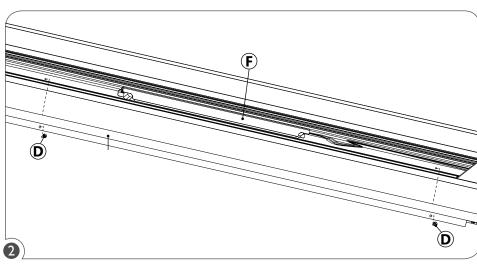
Remove the side reflector retaining screws (D) to access ballast (E).
