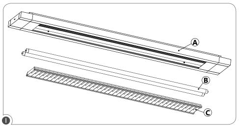
NOTE: Before attempting to verify and replace the ballast, the power to the fixture (A) must be turned off. Disconnect all circuits and remove lamps (B) and optics (C).
