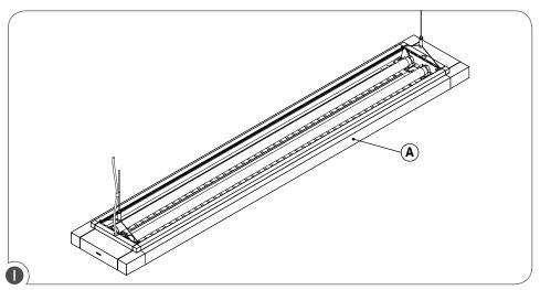
**NOTE:** Before attempting to verify and replace the ballast, the power to the fixture (A) must be turned off. Disconnect all circuits.
