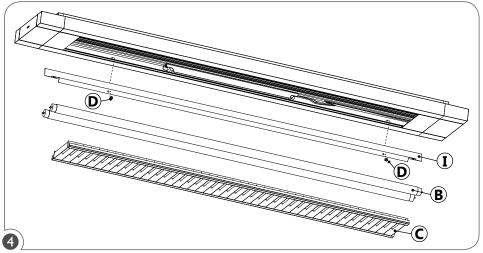
Put the side reflector (I) back in place and fasten retaining screws (D). Re-install the lamps (B) and optics (C).
