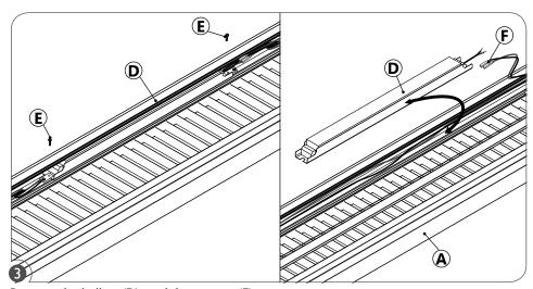
Remove the ballast (D) retaining screws (E) Disconnect wires (F) from the ballast (D). Replace ballast (D) and reconnect wires (F).
