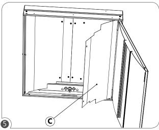
Screw the reflector (C) back into position with a screwdriver.
