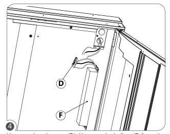
Unscrew the wire nuts (D). Unscrew the ballast (F) from the fixture. Replace the ballast and make connection with wire nuts.
