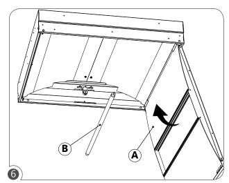
Reinstall the lamps (B) and close the door (A) by snapping back into place.
