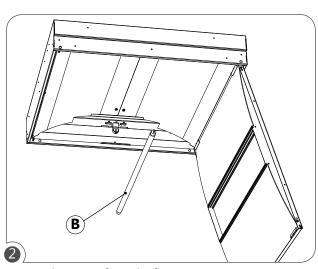
Remove lamps (B) from the fixture.
