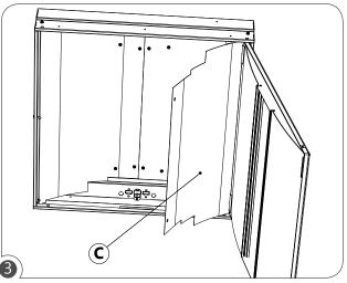
The ballast is always positioned on the hinge side of the door. Unscrew the reflector (C) with a screwdriver.
