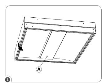
Ensure that the power to the fixture's circuit is turned off. Open the door (A) by pulling down on one side, marked with a white dot, to gain access to the lamps.
