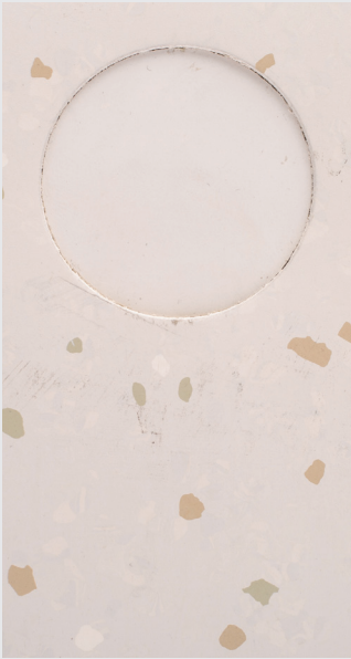
Synthetic Rubber Chip design fades after just 1,600 abrasion cycles
